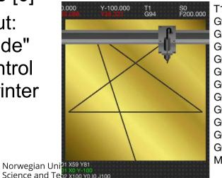
T1 M6 G90 G94 G54 X0 Y0 G00 X0 Y0 G00 X0 Y-100 G01 X-59 Y81 F200 M3 G01 X95 Y-31 G01 X-95 Y-31 G01 X59 Y81 G01 X0 Y-100 G02 X100 Y0 I0 J100 G02 X0 Y-100 I-100 J0 M30;
