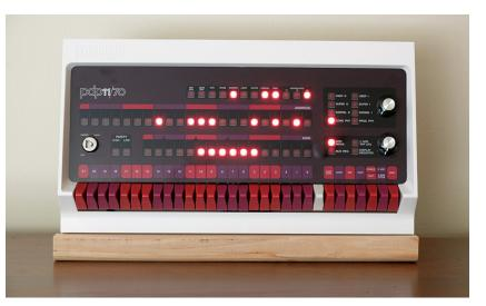
DEC PDP11/70 front panel replica (3D printed) connected to a Raspberry Pi running a PDP11 emulator
