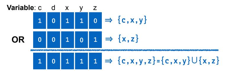
The set property that each element may only occur once in a set is guaranteed by mapping set elements to bits
