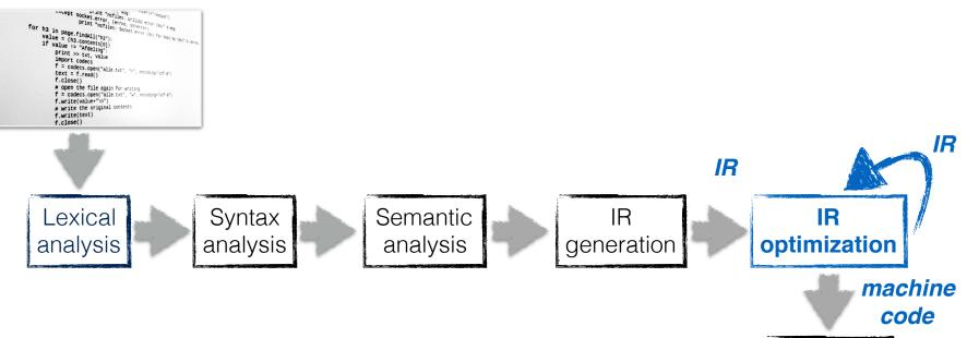
Many analyses and transformations are general (not dependent on the target machine), so they can be easily applied on the **IR level**
