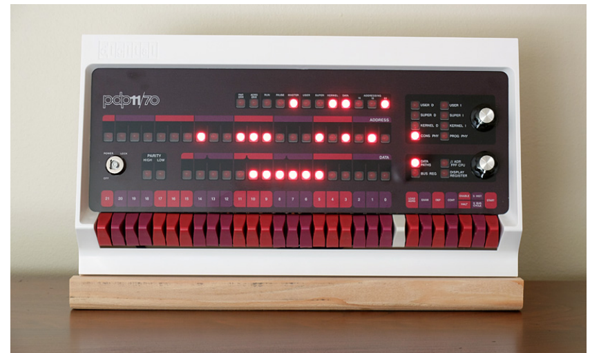
DEC PDP11/70 front panel replica (3D printed) connected to a Raspberry Pi running a PDP11 emulator
